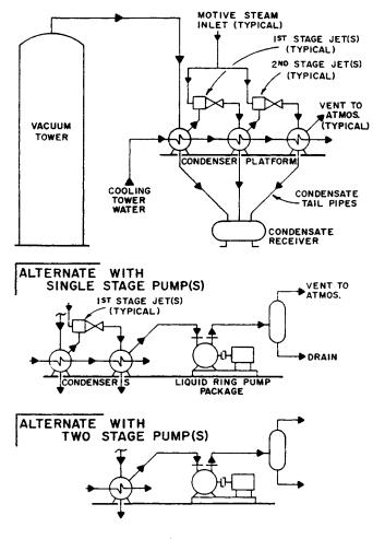
Fig. 2 Typical Schematics
