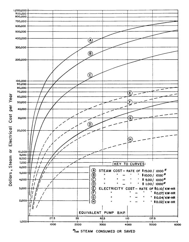
Fig. 6 Steam vs. Electricity Cost
