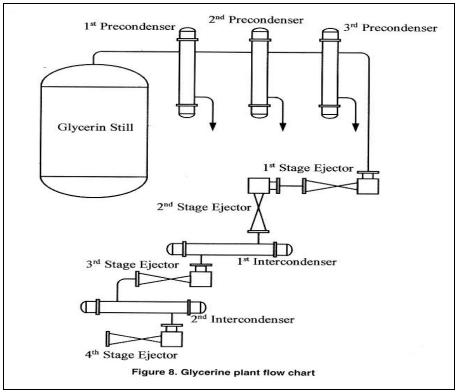
pressure, pressure drop across each precondenser is extremely important. High differential pressure drop not only results in added utilities necessary for the ejector system which backs up the condensers but also reduces the amount of glycerin recovered. The highest value "commercially pure" glycerin production is reduced when pressure drop is high, Furthermore, high pressure drop increases glycerin carryover to the ejector system and as a consequence, increases product loss.
