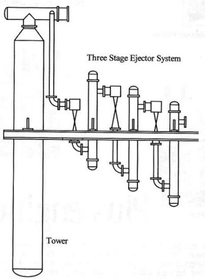
Figure 11. Precondenser mounted atop vacuum column
