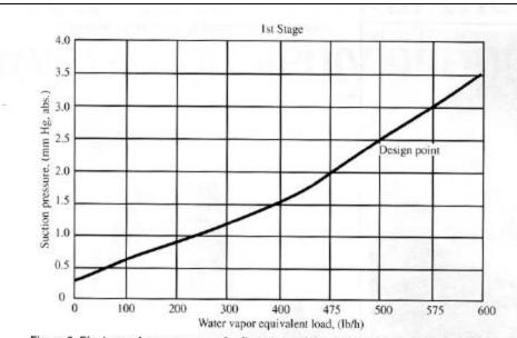
Figure 3. Ejector performance curve for first stage of deodorizer ejector system. (Water vapor equivalent load is on the abscissa and suction pressure maintained by the ejector is shown on the ordinal. Minimum motive steam pressure, 140 psig at 450°F; maximum pressure discharge, 13 mm Hg absolute).
