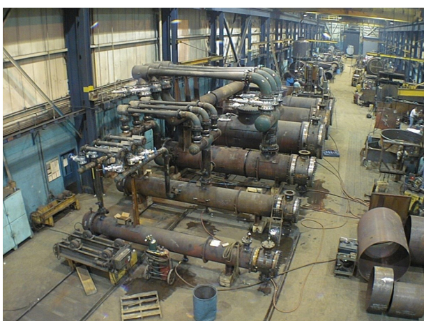
Figure 2. Multiple stage process vacuum condensers with ejectors.
