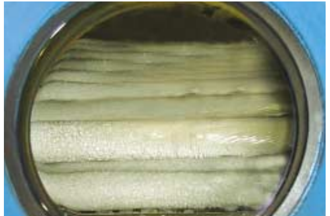
Our freeze condensers trap and solidify product on heat transfer surfaces to improve reclamation and reduce carry-over into the downstream vacuum system.
