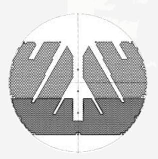
Graham has the knowledge and experience to thermally and hydraulically design and build condensers capable of operating at pressures as low as 0.4 Torr. The above illustrates a tube field layout for a high vacuum process condenser in the production of nylon intermediates.
