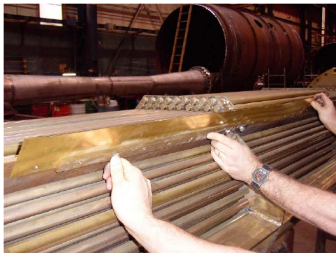
FIG. 1. Sealing strips are utilized to seal to the shell to prevent vapor bypassing.
