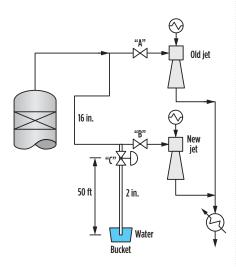
**FIG. 4.** Commissioning the spare first-stage ejector.
