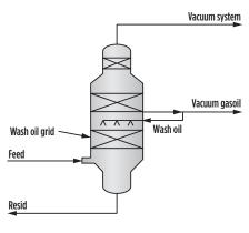
FIG. 2. Wash oil protects the grid from coking.
