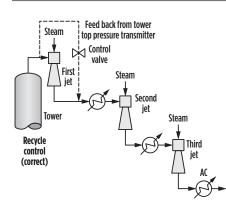
**FIG. 7.** A larger pressure differential allows the sizing of a smaller line and control valve.
