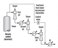
FIG. 6. The vacuum system's recycle pressure control caused the tower pressure to fluctuate when it was put into service, but a P&ID review determined that the recycle line was installed correctly.
