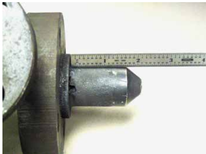
Figure 3. A steam nozzle with a hole through which motive steam leaks into the suction chamber of an ejector. Source: Graham Corporation
