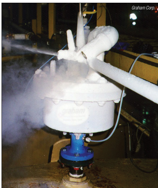
FIGURE 6. Shown here is a cryogenically cooled storage-tank-vent condenser, which prevents the release of vapors into the atmosphere
