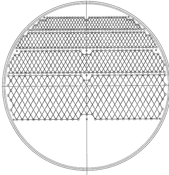
Figure 4. Tube field layout for freeze-condenser that supports 75,000 pph deodorizer
