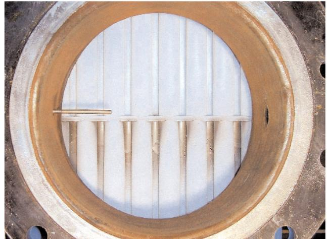
**Figure 3b. End of cycle (when there is substantial ice buildup)**
