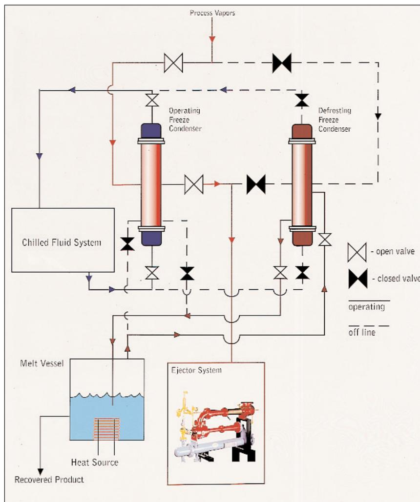
**Schematic of a deodorizer vacuum system utilizing freeze-condensation**
