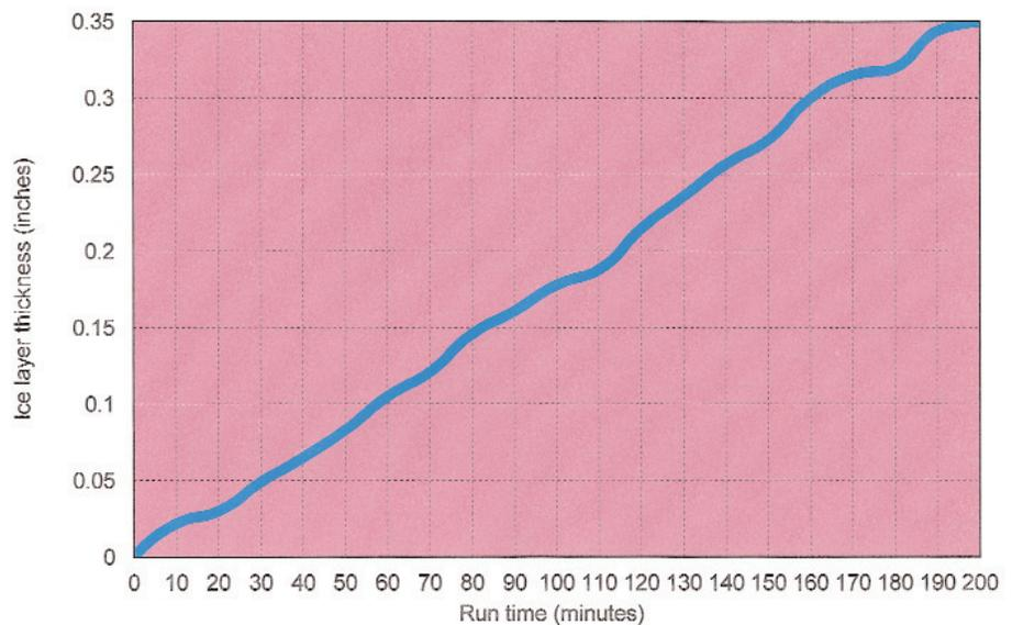
Figure 2. Measured ice thickness vs. time ( $-30^{\circ}\text{F}$  cooling fluid temperature)
