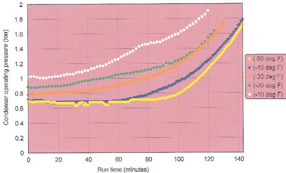
Figure 5. Freeze-condenser performance vs. cooling fluid temperature
