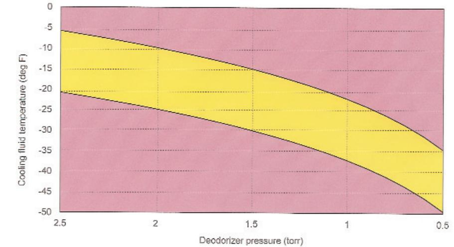
Figure 1. Recommended cooling fluid temperature vs. deodorizer pressure
