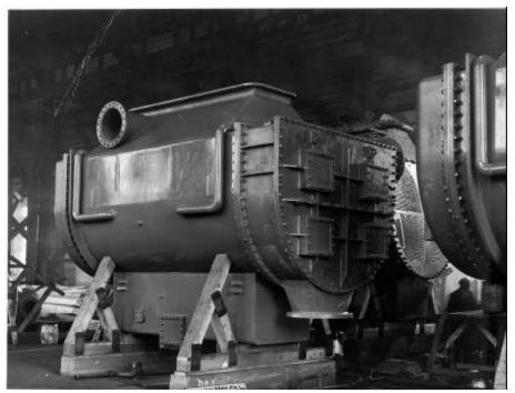
Figure 4 Main surface condenser for T2 tanker ships (1942).
