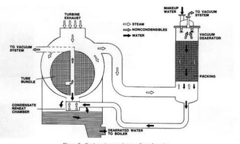
Figure 8 Condenser/vacuum deaerator flow schematic.
