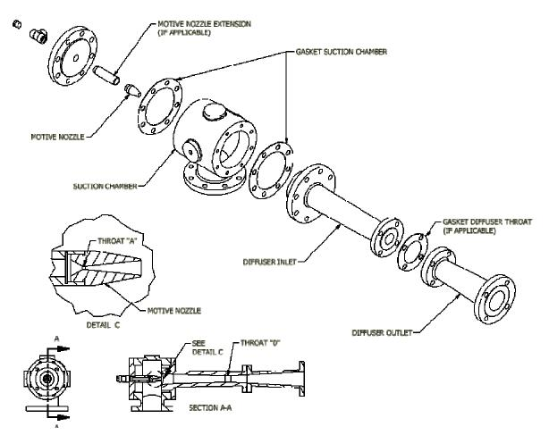
\*Nozzles and diffusers should be replaced when increase in throat area exceeds 7%.
