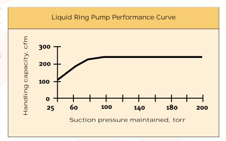
at a constant pressure, while the liquid ring pump is at a lower pressure. The throttle valve is the barrier between the two pieces of equipment that allows each to operate at a different pressure.
