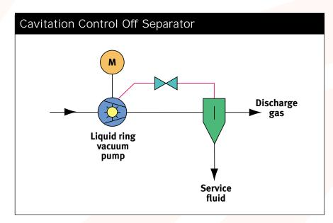
Options for pressure control are similar to those for ejectors. A throttling valve may be used between the vacuum vessel and pump. Again, the valve is a restriction in the line that induces a pressure drop. The pressure vessel operates
