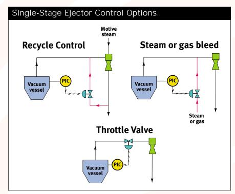
Another means to control pressure when process loading is below design is to introduce an artificial load into the suction line to the ejector. The artificial load can be air, nitrogen, steam or some other gas. Any of these are appropriate for a single-stage ejector. If there is a condenser downstream from the ejector, confirm the condenser will operate with the selected artificial load before beginning.
