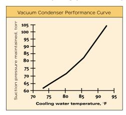
follow the cooling fluid temperature. Recycle control or a steam bleed will not work in this instance. The ejector will not see the recycle or steam bleed because the vacuum condenser has the capacity to condense either of those artificial loads. The recycle stream or steam bleed will go to the condenser and not to the ejector.
