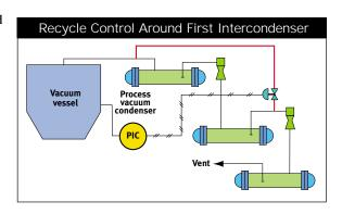
nothing gets added to the process stream. A throttling valve between the process vacuum condenser and first ejector will work as well.
