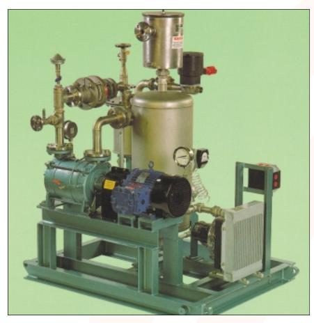
Therefore, an oil sealed liquid ring system can pull to a deeper vacuum than that of a system using water when operating at lower pressures. This also means less of the service liquid will flash, increasing the effective capacity of the vacuum pump.
