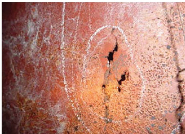
Corrosion can cause holes in an ejector system's diffuser (Fig. 2). Photo from Graham.
