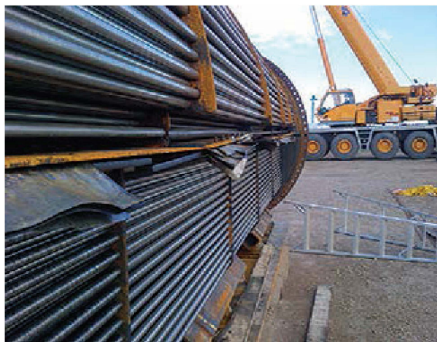
Damaged sealing strips degrade ejector-system performance by allowing process vapors to bypass the condenser (Fig. 4). Photo from Graham.
