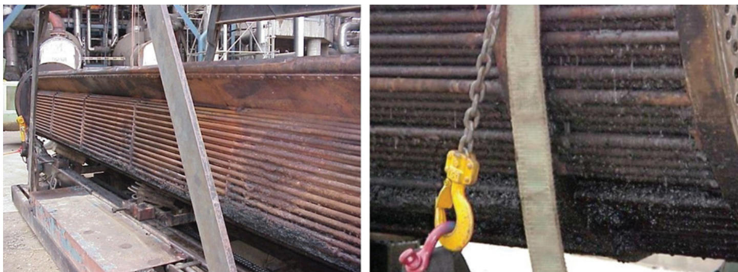
FIG. 3. Shell-side fouling from hydrocarbons in vacuum column overhead loading.
