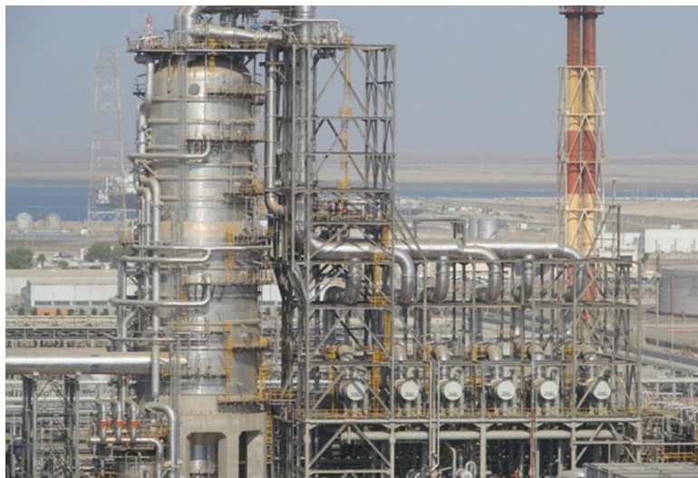
FIG. 2. Vertically mounted first-stage ejectors and piping with expansion loops to address piping stresses that added hydraulic loss between first-stage ejectors and six intercondensers.
