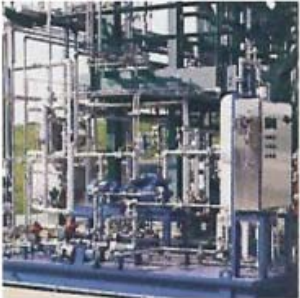
Vacuum pump packaged systems
