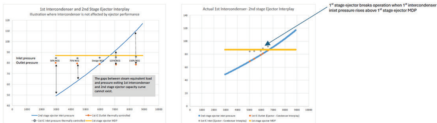
FIG. 2. The first intercondenser and second-stage ejector interplay where the intercondenser is unaffected by the ejector's performance (a), and the actual first intercondenser and second-stage ejector interplay.
